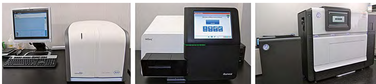
Fig. 2. The next-generation sequencers installed in our department, Roche 454 GS Junior Bench Top System, illumina MiSeq Personal Sequencer, Pacific Biosciences RS System.
