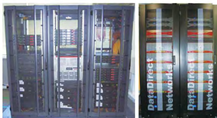
Figure 4. Genome Information Research Center Computer System: Analysis servers (left) and 1.8PB storage system (right).
